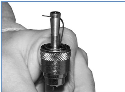
Insert the square-wire from the bottom of the female-adaptor. The phase is helpful to guide the wire. Fold the wire in a angle of 90° and insert them through the upper eyelet.
