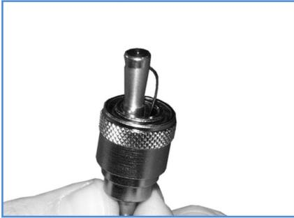
Adjust the rest of the wire to the phase and insert the awl complete into the female adapter, if necessary by using a screwdriver or something like that. The exact fitting will help to connect the part to the male adapter.
