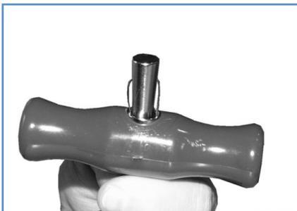
Insert the other end of the wire through the bottom of the safety handle, guide it through the eyelet and fold the wire in a angle of 180°. Close the handle subsequently to fix the wire. By pulling the safety handle the windshield can be easily removed.
