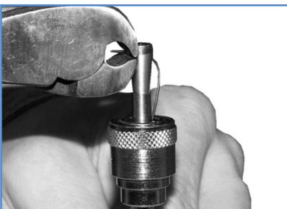
Cut the wire at the level from the eyelet.
